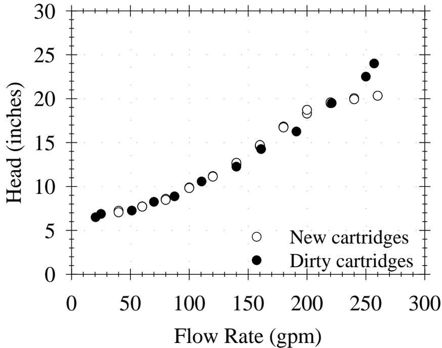
**Figure B3: Hydraulic response of the Jellyfish® Filter JF4-2-1 with clean cartridges prior to commissioning and with dirty cartridges after the monitoring period (25 storm events, 15 inches of cumulative rainfall, 29,851 gallons of treated runoff, and 166 pounds of captured PM mass)**
