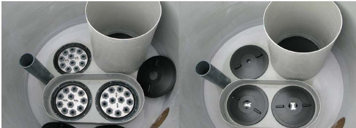
**Figure 7** Top view photos of the Jellyfish<sup>®</sup> Filter JF4-2-1 deck with two hi-flo cartridges and one draindown cartridge installed with cartridge lids off (upper left image) and cartridge lids on (upper right image). The backwash pool weir encloses the hi-flo cartridge. Also shown are the maintenance access pipe (large), pressure relief pipe (small), and the outlet opening (lower right in each image).
