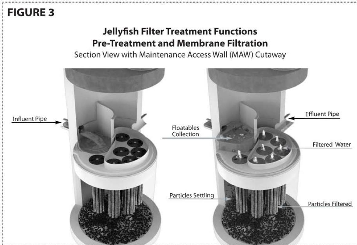
Pre-treatment removes coarse sediment (particles generally > 50 microns), particulate-bound pollutants attached to coarse sediment (nutrients, toxic metals, hydrocarbons), free oil and floatable trash and debris. These pollutants are removed by gravity separation. Large, heavy particles fall to the sump (sedimentation) and low density pollutants rise to the surface (floatation) within the pre-treatment channel.
