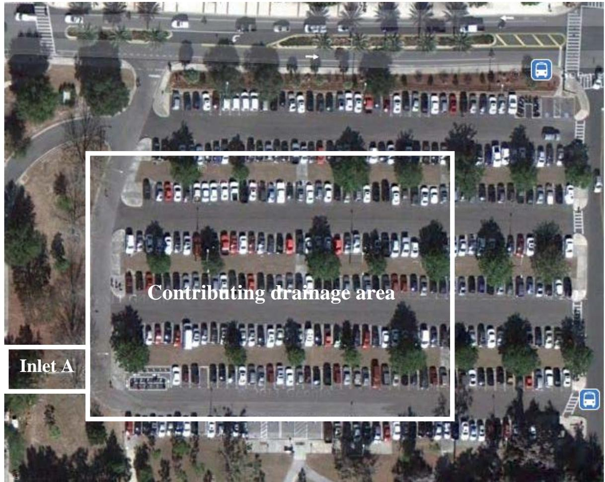
Depending on the storm event intensity and wind direction the drainage area can vary from 5,400 to 8,600 ft<sup>2</sup> (0.12 to 0.20 acres) of pavement. The catchment drains to inlet A as shown in Figure 4(b) and 4(a). Runoff captured by inlet A is the source of influent to the downstream Jellyfish Filter.
