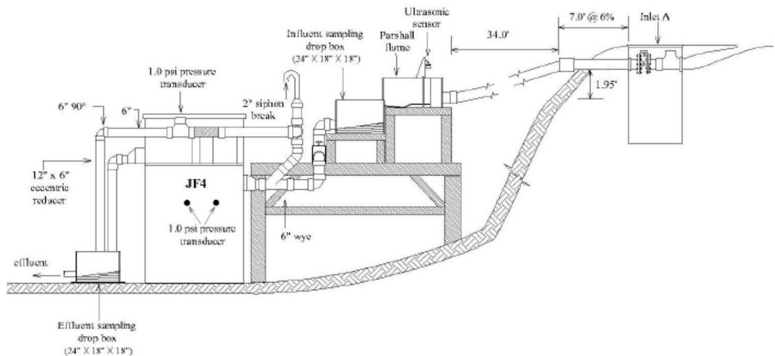
**Figure 5 Profile view schematic of the field set-up for the Jellyfish<sup>®</sup> Filter JF4-2-1**
