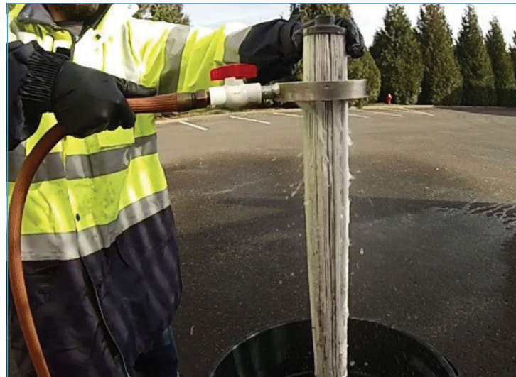
The Jellyfish Filter cartridge is light and easy to clean.
